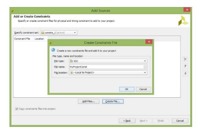
This returns to the Add or Create Constraints so multiple files can be added at the same time. Only 1 file is needed for this example, so click Finish
