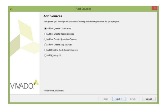
Just as before with the VHDL module, a previously created constraints file could be added to the project by clicking Add Files. To create a new file, click Create File
