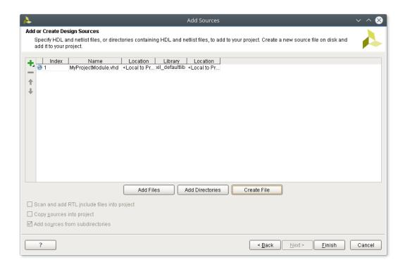
After all of the wanted sources have been added, click Finish. This will bring up a Define Module dialogue box to create a framework for each of the VHDL modules. With this dialogue, each module can have the inputs and outputs defined. For this project, A, B, C, and D are inputs (in) and X, Y, and Z are outputs (out).
