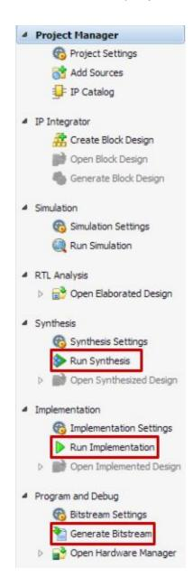
Each process can be run individually by double clicking on them or right clicking and selecting Launch. If you double click on a process that requires a previous process that has not already been run, the prerequisite processes will be run automatically.
